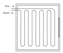
Once the pipework has been laid, work out where to cut the pipe for the final connection into the manifold (ensure this will not be too short for the manifold connection). Insert into the final compression fitting and connection on to the manifold. Tighten the compression fittings after this.
