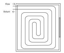
Serpentine pipe layout for odd shaped or specific heat areas (i.e. to concentrate flow near windows or doors)
