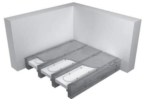
Cover the pipe with 25mm-50mm screed
