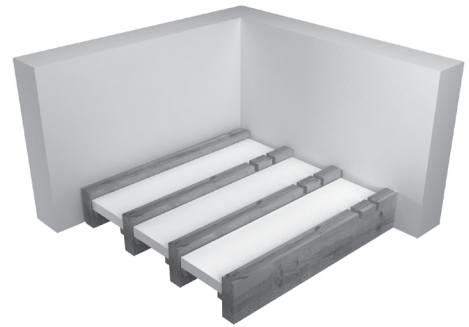
Fit insulation between the joists
