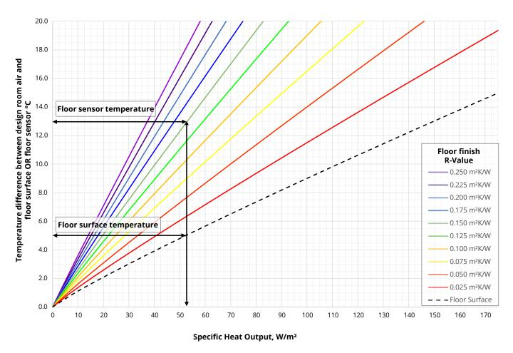
Using the graph above it is possible to get the specific heat output of an eUFH system based on the temperature difference between the design room air temperature and the floor surface or floor sensor temperature by floor finish.
